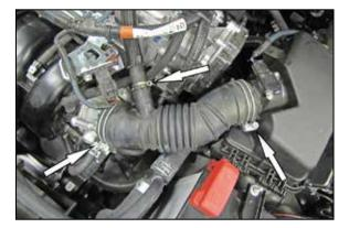
3. Loosen the hose clamps securing the intake tube and release the spring clamp on the crank case vent hose. Disconnect the crank case vent hose and then remove the factory intake tube from the vehicle.
