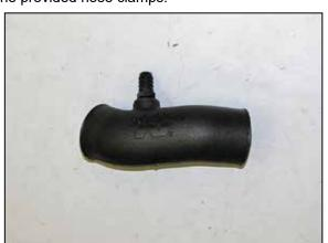
6. Install the provided crank case vent fitting into the  $K\&N^{@}$  intake tube as shown.
