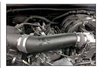
12. Adjust the intake tube for best fit and then secure with the provide hose clamps.
