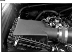
11. Reinstall the factory air filter housing and secure with the factory retaining clips.
