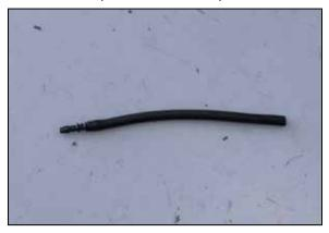
13. Install the hose mender into the provided fuel pressure regulator hose as shown.
