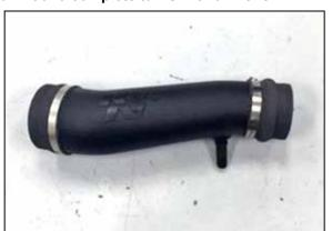
9. Install the provided coupler hoses onto the K&N® intake tube as shown and secure with the provided hose clamps.
