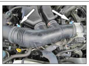
5. Loosen the two hose clamps that secure the intake tube assembly to the throttle body and air filter housing.
