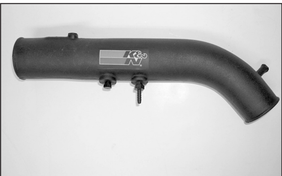
12. On 03 models, install provided vent and plug into the K&N® intake tube as shown.
