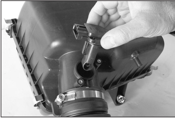
8. Loosen and remove the screws that secure the mass air sensor, then remove the mass air sensor.
