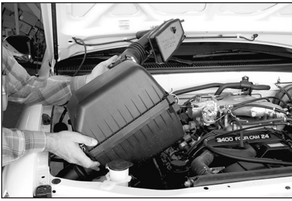
7. Remove the complete air intake system. NOTE: K&N Engineering, Inc., recommends that customers do not discard factory air intake.
