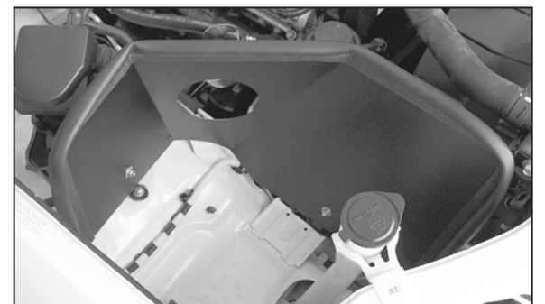
20. Install the heat shield and secure it to the new K&N® brackets with the hardware provided. Do not tighten completely.
