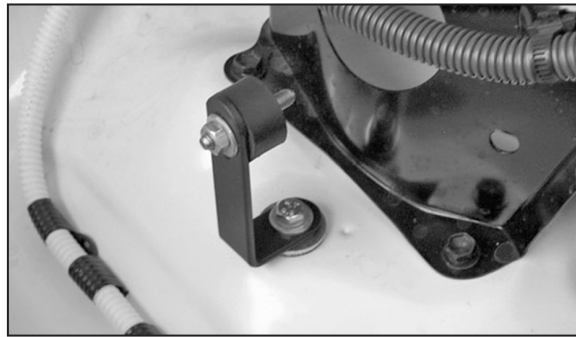
15. Install the "L" bracket onto the existing air box-mounting hole. NOTE: Rubber washer & fender washer should be mounted between the fender and the bracket. Do not tighten completely.
