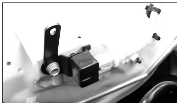
18. Install the bracket onto the relay bracket using the bolt that was removed in step 17. Do not tighten completely.
