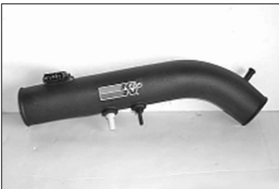
11. On 2000-02 models, install provided vents into the K&N® intake tube as shown. NOTE: Plastic NPT fittings are easy to cross thread. Install the vent fitting "hand" tight, then turn it two complete turns with a wrench.
