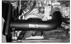
22. Install the new air intake tube to the throttle body and heat shield then tighten the hose clamps.
