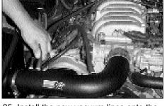
25. Install the new vacuum lines onto the new intake tube as shown.
