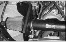
27. Install the new K&N® Air Filter onto the new air intake tube.
