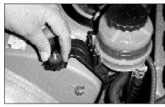
19. Install the rubber studs to the stock air box mounting location as shown.
