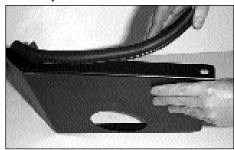
17. Install the edge trim to heat shield as shown.
