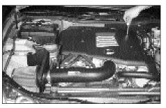
29. Install the engine cover back onto the motor and tighten the four bolts.
