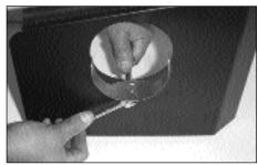
18. Install the saddle bracket assembly to the heat shield as shown.
