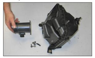
2. Depress the locking tab and disconnect the mass air sensor electrical connection. Next separate the mass air sensor wire harness from the clips, which attach to the air box.
