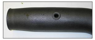
15. Install the provided grommet into the K&N $^{\mbox{\tiny \$}}$  intake as shown.
