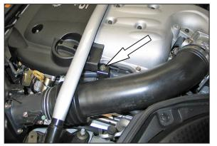
3. Remove the bolt, which secures the stock intake tube to intake manifold. NOTE: Do not discard this bolt, as it will be used in a later step. 5. Remove the air box mounting bolt, which secures the air box to the inner fender.
