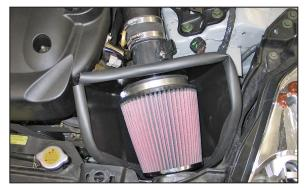
21. Install the Air Filter / mass air sensor assembly onto the K&N<sup>®</sup> intake tube, slide the silicone hose onto the mass air sensor housing and secure with the provided hose clamp as shown.
