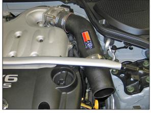
18. Install the K&N<sup>®</sup> intake tube onto the throttle body and saddle clamp and then secure with the provided hose clamps as shown.
