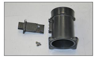
9. Remove the two screws, which secure the mass air sensor into the mass air housing, then remove the mass air sensor from the housing. **NOTE: Do not discard the mounting screws, as they will be reused in a later step.**
