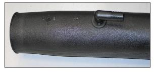
16. Install the provided 90 deg. fitting into the grommet that was installed onto the K&N<sup>®</sup> intake tube in step #15.
