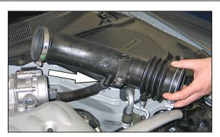
4. Loosen the two hose clamps, which secure the stock intake tube to the throttle body and air box. Then lift the intake tube up to access the crank case vent hose and disconnect the vent hose from the intake tube. Next remove the intake tube from the vehicle.
