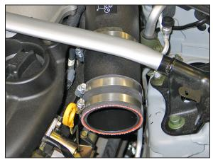
19. Install the silicone hose (08690) onto the end of the K&N<sup>®</sup> intake tube with the provided hose clamps.
