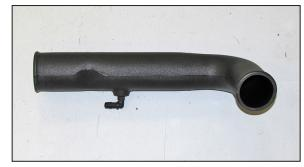
8. Install the provided vent fitting into the K&N<sup>®</sup> intake tube as shown.
