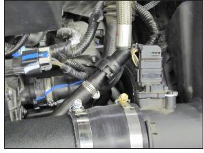
14. Connect the factory crank case vent fitting into the K&N<sup>®</sup> quick connect fitting as shown.
