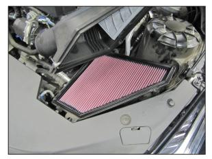
7. Install the K&N<sup>®</sup> air filter and then secure the lid with the factory hardware.
