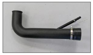
11. Install the provided step coupler (08429) onto the K&N^ $\ensuremath{\mathbb{S}}$  intake tube.
