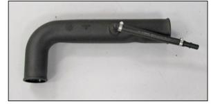
10. Install the crank case vent assembly onto the fitting installed into the K&N<sup>®</sup> intake tube and secure with the provided hose clamp.
