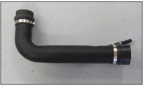
12. Install the provided hump coupler (08185) onto the K&N $^{\circ}$  intake tube as shown and secure with the provided hose clamp.
