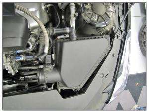
6. Loosen the four screws securing the air box lid and then remove the factory air filter.
