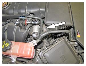
4. Loosen the hose clamp securing the intake plenum to the throttle body.
