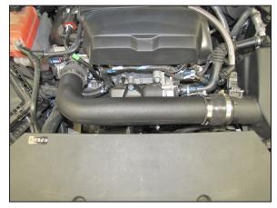
13. Install the K&N<sup>®</sup> intake tube assembly onto the air box and then onto the throttle body. Adjust the tube and coupler for best fit and then secure with the provided hose clamps.
