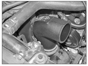
9. Install the new K&N $^{\odot}$  intake tube onto the intake track and secure with the provided hose clamps.
