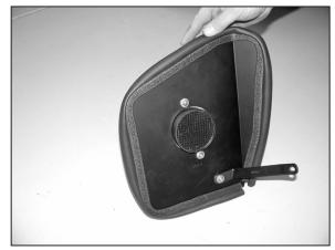
12. Attach the bracket onto heat shield with the provided hardware as shown.
