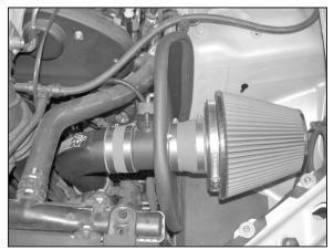
17. Install the K&N<sup>®</sup> filtercharger onto the mass air assembly as shown.
