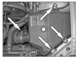
3. Loosen hose clamp at the mass air, then remove the three 10mm bolts that secure air box to vehicle.
