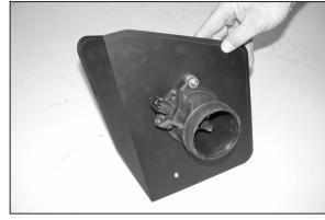
10. Install the mass air sensor onto the heat shield with the provided spacers and hardware as shown.
