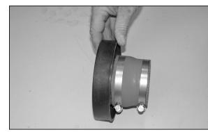
15. Install the silicone hose (08051) onto the filter adapter as shown.
