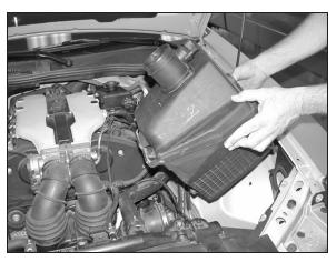
4. Remove air box from vehicle as shown.
