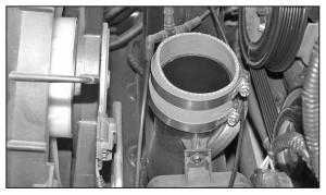
8. Install silicone hose (08434) onto intake track with the provided hose clamps as shown.
