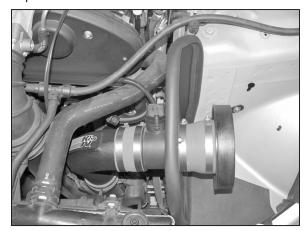
16. Install the filter adapter onto the mass air sensor with the provided hose clamps.
