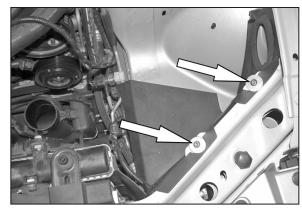
6. Secure splash shield onto vehicle with the provided hardware as shown.
