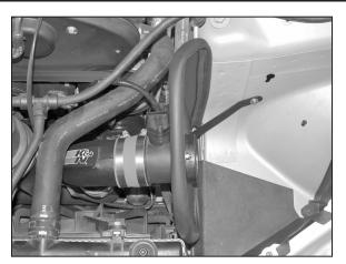
14. Install the heat shield assembly onto the vehicle, then attach intake tube to silicone hose and secure bracket to wheel well as shown.
