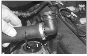
20a. On vehicles with air injection cut the vent hose 1" from end of hose.
