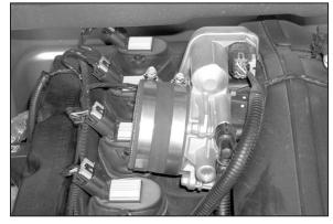
15. Install the silicone hose onto the throttle body with the provided hose clamps.
