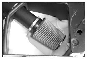
24. Install the K&N<sup>®</sup> Air Filter onto the K&N<sup>®</sup> intake tube as shown.
