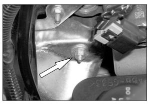
13. Remove the nut that secures the exhaust heat shield to cylinder head as shown.
