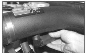
12. Assemble the saddle bracket assembly as shown.
