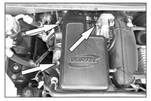
8. Loosen the two bolts that retain the intake resonator and then loosen the hose clamp at the throttle body.
