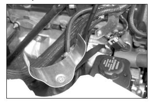
14. Using the nut that was removed in the previous step, install the saddle bracket as shown.
