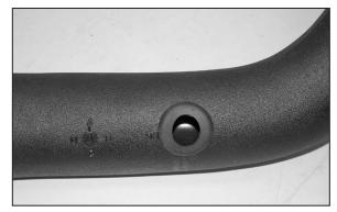
20c. Use a 1-1/4 hole saw and drill a hole where the intake tube was marked in the previous step. Then install the provided grommet as shown.
