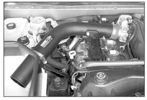
20. Install the new K&N<sup>®</sup> intake tube into the vehicle and tightening hose clamp at the throttle body and at the saddle bracket as shown.
