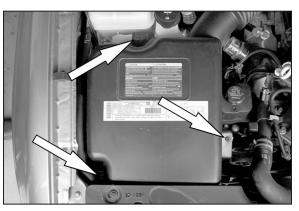
3. Loosen and remove the three screws that retain the upper airbox cover.
