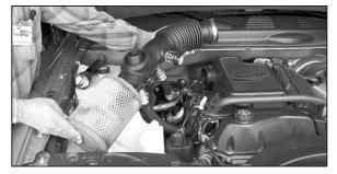
2. On vehicles equipped with a fuel pressure regulator vent, diconnect the vent hose form the fuel pressure regulator as shown.
