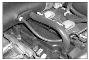
22. Install the 1/2" silicone hose onto the K&N $^{\odot}$  intake tube and the other end onto the crankcase vent as shown.
