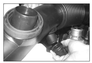
5a. On vehicles with air injection squeeze release ring then remove air injection line from intake tube.
