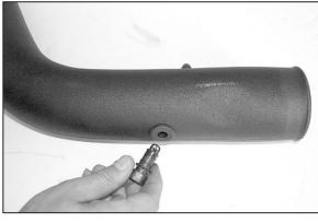
19. Install the air temp sensor into the new  $K\&N^{\mbox{\scriptsize \$}}$  intake tube as shown.
