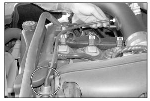
21. On Vehicles eqipped with a fuel pressure regulator vent hose, install the provided 4mm silicone hose onto the K&N<sup>®</sup> intake tube and the other end onto the fuel pressure regulator vent as shown.
