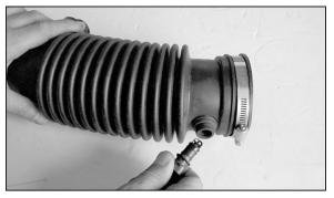
17. Remove the air temp sensor from stock intake tube as shown.
