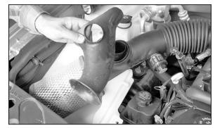
5. Remove the fresh air supply tube from vehicle.
