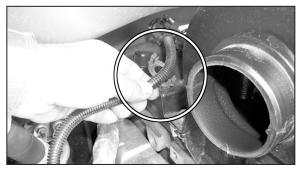
7. Disconnect the clip that holds the air temp. electrical connection wiring loom then remove the wire loom.
