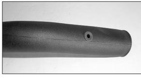
18. Install the provided grommet onto the new  $K\&N^{\circledast}$  intake tube as shown.
