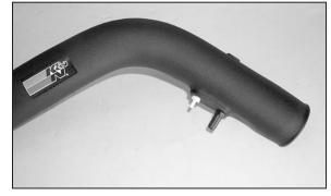
16. Install the provided vent fittings onto the  $K\&N^{\otimes}$  intake tube as shown.
