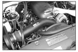
12. Install the K&N<sup>®</sup> intake tube onto the mass air sensor, then secure the other end onto the throttle body as shown.
