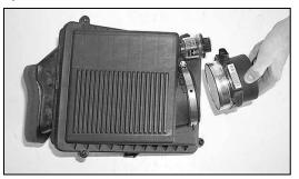
6. Loosen the hose clamp and remove the mass air sensor from the air cleaner.
