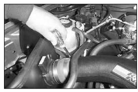
28. Tighten the hose clamp on the silicone hose at the intake tube.
