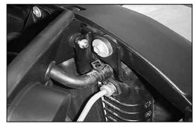
22. Secure the rubber mounted stud to the radiator mounting bracket.
