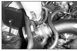
26. Align the intake tube with the mass air sensor and tighten the hose clamp on the silicone hose at the mass air sensor.
