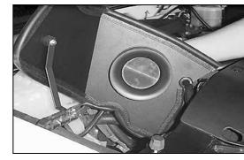
20. Install the heat shield assembly.
