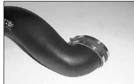
23. Install the 4"ID silicone hose onto the intake tube.
