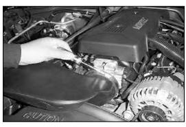
4. Loosen the hose clamp on the intake tube at the throttle body.
