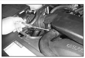
5. Using a flat blade screwdriver, pry the radiator hose retaining clip from the intake tube.
