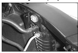
16. Measure over and down ½" on the radiator mounting bracket and mark.
