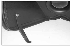
15. Attach the bracket assembly to the heat shield using the hardware provided.
