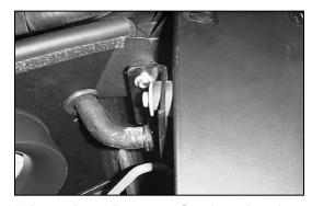
30. Insert the radiator over flow hose into the grommet on the heat shield.
