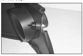
18. Attach a rubber mounted stud to the heat shield using the hardware provided.
