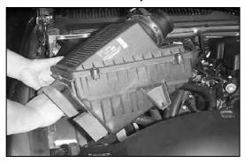
8. Pull firmly upward and remove the airbox. NOTE: K&N Engineering, Inc., recommends that customers do not discard factory air intake.
