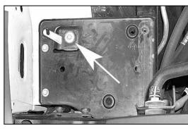
19. Loosen and remove the bolt from the airbox mounting tray.
