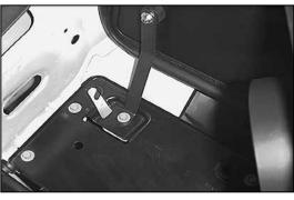
21. Secure the bracket to the airbox mounting tray using the bolt removed in step 19.
