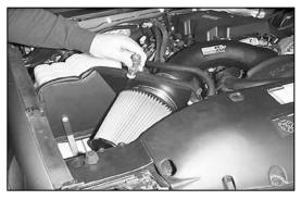
32. Install the air filter and secure with hose clamp.
