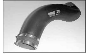
24. Install the 3.75"ID silicone hose (08631) onto the intake tube.
