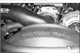
31. Due to production tolerances it may be necessary to mark the fan shroud as indicated, remove the intake tube and trim the fan shroud. NOTE: Be sure to cover the throttle body and alternator during this process.
