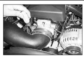
25. Install the intake tube and tighten the hose clamp on the silicone hose at the throttle body.
