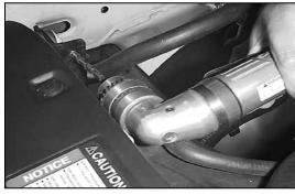
17. Using  $\frac{1}{4}$ " drill bit, drill out location marked in the previous step.
