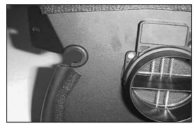
14. Install the grommet onto the heat shield.
