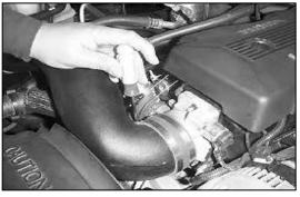
27. Align and check the intake tube for clearance, tighten the hose clamp on the silicone hose at the intake tube.
