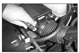
3. Loosen the hose clamp on the intake hose at the mass air sensor.
