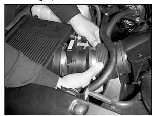
6. Detach the intake hose from the mass air sensor.
