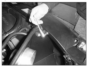
20. Secure the "L" bracket to the threaded hole in the radiator core support using the hardware provided.
