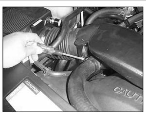
5. Using a flat blade screwdriver, pry the radiator hose retaining clip from the intake tube.
