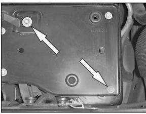
16. Loosen and remove the two bolts on the airbox mounting tray.
