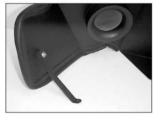
13. Attach the "C" bracket assembly to the heat shield as shown.
