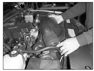
7. Detach the intake tube from the throttle body and remove the intake assembly.
