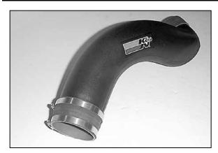
23. Install the 3.75"ID silicone hose (08631) onto the intake tube.
