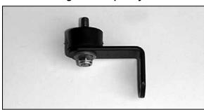
14. Attach the rubber mounted stud to the "L" bracket.
