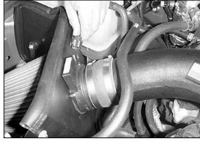
31. Reconnect the mass air sensor electrical connector.
