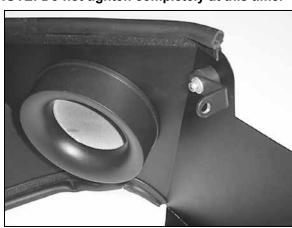
15. Attach the "L" bracket assembly to the heat shield.
