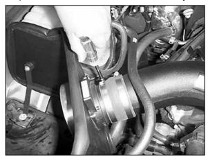
25. Align the intake tube with the mass air sensor and tighten the hose clamp on the silicone hose at the mass air sensor.
