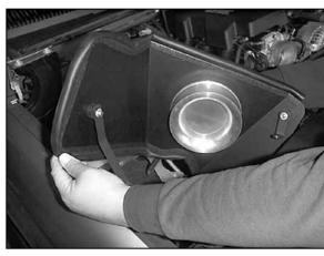
18. Install the heat shield assembly.
