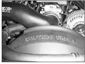
29. Due to production tolerances it may be necessary to mark the fan shroud as indicated, remove the intake tube and trim the fan shroud. NOTE: Be sure to cover the throttle body and alternator during this process.
