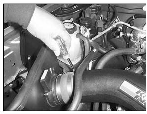
27. Tighten the hose clamp on the silicone hose at the intake tube.
