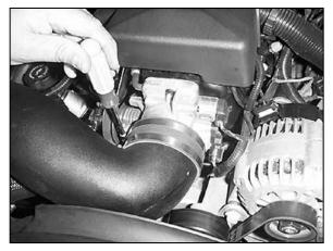
24. Install the intake tube and tighten the hose clamp on the silicone hose at the throttle body.
