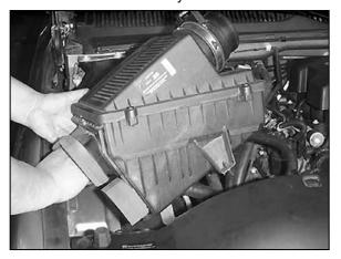
8. Pull firmly upward and remove the airbox.
