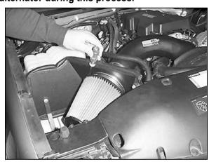
30. Install the Air filter element and secure with hose clamp.
