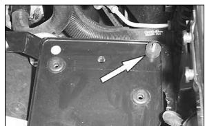
17. Install the rubber mounted stud into the threaded hole in the airbox mounting tray as shown.
