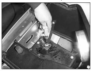
19. Secure the "C" bracket to the threaded hole in the airbox mounting tray using the bolt removed in step 16.
