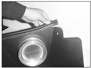
11. Install the trim seal onto the heat shield as shown.
