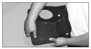
13. Insert the grommets provided, into the holes onto the bottom side of the heat shield.
