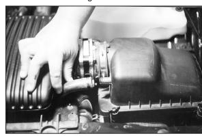
5. Detach the air injection hose from the airbox.
