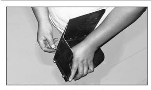
11. Assemble the heat shield by using nylock nuts and allen head bolts provided.
