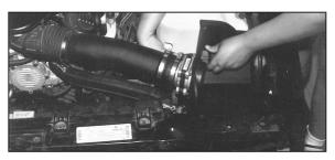
23. Insert the air filter through the hole in the heat shield. connect the air injection hose to the air filter and secure with hose clamp.
