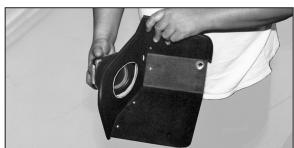
15. Install the mass air sensor into the hole in the heat shield.
