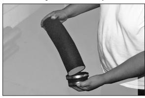
20. Install the hose clamps on the tube adapter and install this assembly onto the intake tube.
