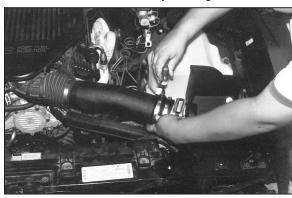
22. Install loose end of intake tube on mass air sensor and tighten all hose clamps.
