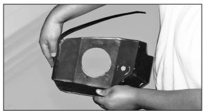
12. Install trim seal on edge of heat shield. NOTE: Some trimming may be necessary for the best fit.
