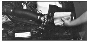
24. Install the air filter element with hose clamp and tighten.
