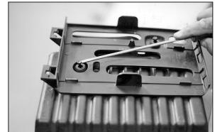
9. Remove the computer cover from the lower airbox housing.
