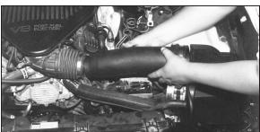
21. Install intake tube assembly by pushing end into rubber bellows assembly on engine.
