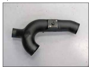
20. Install the inlet air temperature sensor assembly into the  $K\&N^{@}$  intake tube and secure with the provided hardware.
