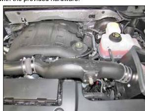
21. Install the K&N® intake tube into the coupling hoses and then secure with the provided hose clamps.
