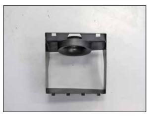
5. Install the provided filter adapter into the heat shield and secure with the provided hardware.
