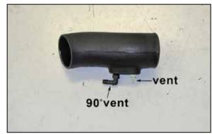
9. Install the provided 1/4npt vent fittings into the  $K\&N^{\otimes}$  intake tube as show.
