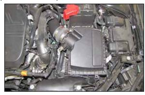
17. Install the upper air box and Intake tube and then secure the air box with the factory clips. Adjust the intake tube for best fit and then secure it with the hose clamps provided to the two hump hoses.
