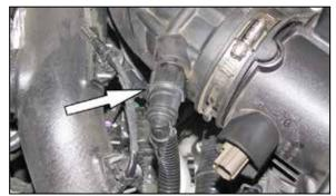
3. Disconnect the crank case vent connection.
