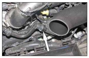
14. Connect the factory crank case vent hose to the quick connect fitting/vent hose installed into the K&N<sup>®</sup> intake tube.
