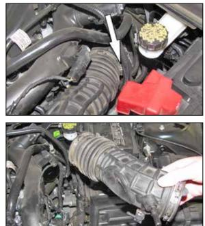
2. Disconnect the Inlet air temperature sensor electrical connection.
