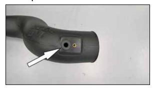
12. Install provided grommet into K&N® intake tube. NOTE: On vehicles equipped with the sensor without the bolt to secure it will need the hole in the intake tube drilled out to ¾"id and use supplied grommet #08064.
