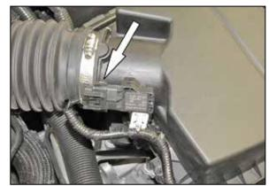
6. Disconnect the temperature sensor electrical connect.
