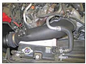
31. Install the intake tube into the silicone hose attached to the filter adapter and align the tube with the factory intake. Slide the silicone hose onto the factory intake and the secure the tube with the hose clamps.
