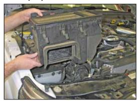
11. Remove the lower air box from the vehicle. NOTE: K&N Engineering, Inc., recommends that customers do not discard factory air intake.
