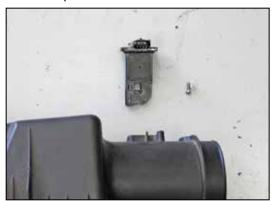
27. Remove the two screws securing the mass air sensor into the factory air box and then remove the sensor from the air box.
