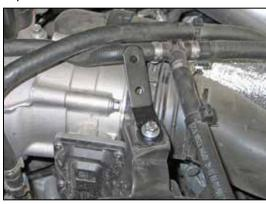
33. Install the coolant hose bracket onto the fan shroud as shown using the provided hardware.
