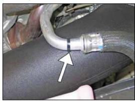
32. Secure the coolant pipe to the insert of the K&N® intake tube with the provided mounting tie wrap.
