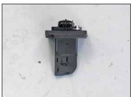
28. Install the mass air sensor into the K&N® mass air sensor adapter and secure with the provided hardware.
