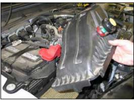
5. Remove the upper air box housing from the
