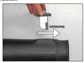
29. Install the mass air sensor assembly into the  $K\&N^{@}$  intake tube as shown and secure with the provided hardware.
