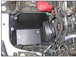
24. Set the heat shield assembly into position and secure with the factory mounting hardware from step #12.
