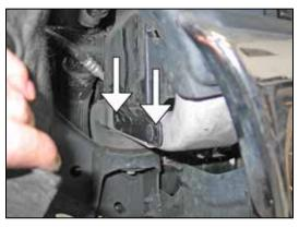
16. Remove the two clips shown that retain the bottom of the fresh air intake duct.
