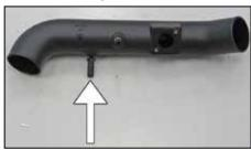
17. Install the provided quick disconnect fitting into the K&N® intake tube as shown.
