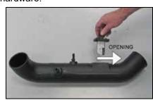
21. Install the mass air sensor assembly into the K&N® intake tube and secure with the provided hardware.
