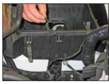
12. Remove the center airbox retaining clip.
