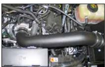
22. Install the K&N® intake tube assembly into the silicone hose at the filter adapter and then into the silicone hose on the throttle body and secure with the provided hose clamps.
