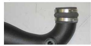
21. Install the provided silicone (087121) hose onto the K&N<sup>®</sup> intake tube with the hose clamps provided as shown.
