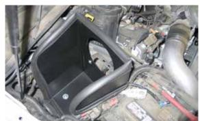
13. Install the heat shield assembly into position so that the rubber mounted studs protrude through bottom of the heat shield. Secure the heat shield with the provided hardware and the factory battery tray bolt removed in step #12.
