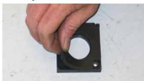
18. Install the provided gasket onto the K&N® mass air sensor adapter.
