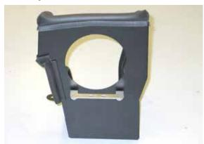
9. Install the tube mounting bracket (06712) onto the heat shield using the provided hardware and spacers.
