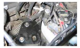
12. Remove the battery tray mounting bolt shown. **NOTE: This bolt will be reused.**
