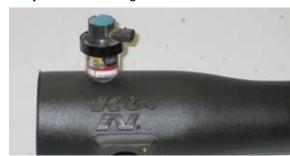
15. Install the filter minder and grommet into the K&N® intake tube as shown.
