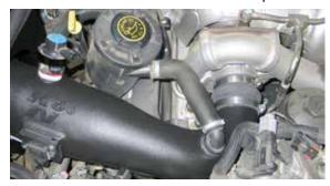
23. Insert the crank case vent fitting into the grommet in the  $K\&N^{\mbox{\tiny @}}$  intake tube.
