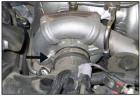
5. Loosen the hose clamp which secures the intake tube to the turbo inlet.
