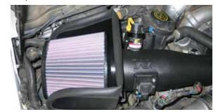
25. Install the K&N® Air Filter onto the K&N® intake tube and secure with the hose clamp.
