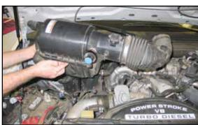
7. Lift up firmly on the complete air box assembly to dislodge it from the mounting grommets and then remove the complete air box and intake tube assembly from the vehicle.
