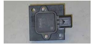
19. Install the mass air sensor into the K&N® mass air sensor adapter and secure with the provided hardware.
