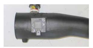
20. Install the mass air sensor assembly onto the K&N® intake tube as shown and secure with the provided hardware as shown.
