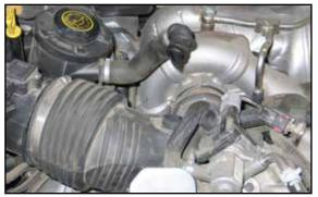
4. Clip the band clamp which secures the crank case breather hose to the intake tube. Then disconnect the breather hose and fitting from the intake tube as shown.
