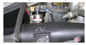
24. Attach the filter minder extension harness provided into the factory harness and then connect the open end to the filter minder.
