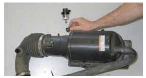
14. Remove the filter minder and grommet from the factory air filter housing as shown.
