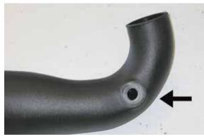
16. Install the supplied crank case grommet into the K&N® intake tube as shown.
