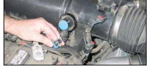
3. Disconnect the filter minder electrical connection.
