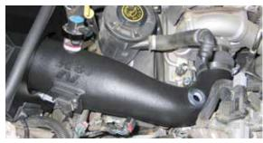
22. Install the K&N® intake tube assembly into the heat shield and slide the silicone hose onto the turbo inlet. Secure the intake tube to the mounting bracket on the heat shield with the provided hardware and then position the silicone hose onto the turbo and secure with the hose clamps.
