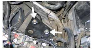
11. Install the provided rubber mounted studs onto the heat shield mounting tray using the provided hardware
