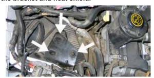
10. Remove the three air box mounting grommets shown from the mounting tray.
