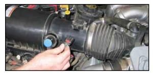
2. Disconnect the mass air sensor electrical connection and unclip the wiring harness from the air box as shown.
