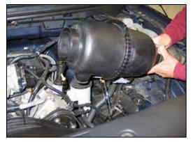
4. Firmly pull up the assembly to unhook it from the mounting grommets and inner fender as shown. NOTE: Use caution as the mass air sensor electrical harness will still be connected. NOTE: K&N Engineering, Inc., recommends that customers do not discard factory air intake. 5. Unhook the secondary mass air sensor connection from the clip that secures it to the air box mounting bracket, then disconnect the secondary mass air connection.
