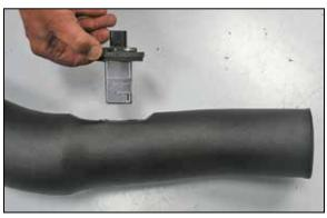
14. Install the mass air sensor assembly into the K&N® intake tube as shown with the opening pointed towards the filter end of the tube.
