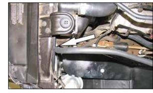
22. Secure the heat shield to the core support with the factory mounting bolts removed in step #10 as shown.
