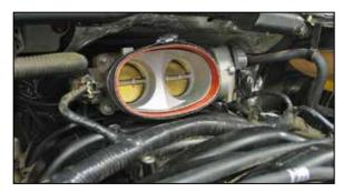
24. Install the silicone hose (08627) onto the throttle body and secure with the provided hose clamp.
