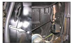
23. Reinstall the support rod with the factory mounting bolts removed in step #8 as shown.
