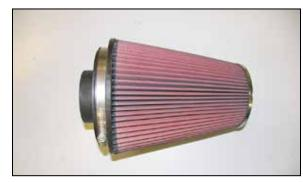
30. Install the filter adapter into the Air filter and secure with the provided hose clamp.
