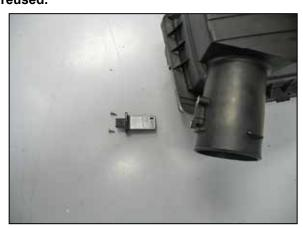
11. Remove the two mass air sensor mounting screws with the T20 TORX wrench provided and then remove the sensor from the air box as shown.
