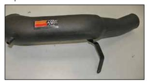
25. Install the tube mounting bracket (26624) onto the K&N® intake tube and secure with the provided hardware as shown.
