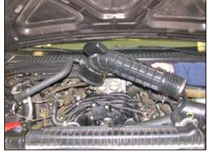
4. Loosen the hose clamps, which secure the intake tube to the throttle body and to the air box, then remove the intake tube from the vehicle.
