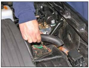
5. Remove the intake air bypass hose from the inner fender as shown.
