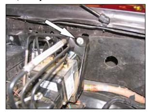
9. Remove the top front ABS brake pump mounting bracket bolt shown.
