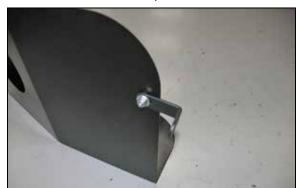
16. Install the small "L" bracket (070812A) onto the heat shield as shown using the provided hardware.
