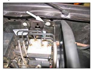
21. Place the rear heat shield bracket between the inner fender and the ABS pump mounting bracket and secure with the factory mounting bolt removed in step #9.
