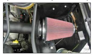
32. Install the air filter assembly onto the K&N® intake tube and secure with the provided hose clamp.
