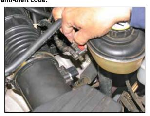
2. Release the red locking tab on the mass air sensor electrical connector and then disconnect the mass air sensor electrical connection and unhook the wiring harness retainer from the intake tube.
