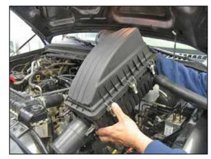
6. Pull up on the rear of the air box assembly to dislodge it from the mounting grommets and then remove the air box from the vehicle.
