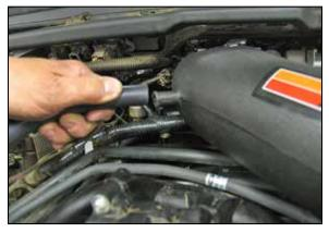
29. Install the crank case vent hose onto the K&N® intake tube as shown.
