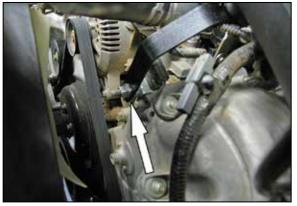
27. Secure the tube mounting bracket to the 8mm stud with the nut and washer provided. Align the K&N® intake tube for best fit and then tighten the hose clamp and bracket mounting hardware.
