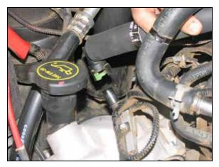
3. Rotate the green locking tab on the crank case vent connector at the valve cover counter clockwise and then pull up and disconnect the crank case vent as shown.
