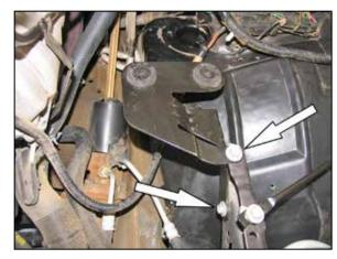
7. Remove the two bolts, which secure the air box mounting bracket shown, and then remove the airbox mounting bracket.
