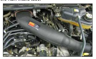
26. Install the K&N® intake tube onto the throttle body and align the mounting bracket so that it sits on the 8mm stud protruding from the cylinder head.
