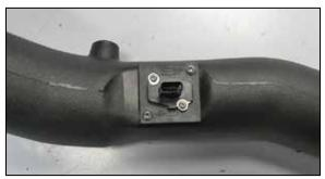
15. Secure the mass air sensor assembly into the  $K\&N^{\circ}$  intake tube with the provided hardware.
