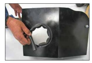
18. Install the edge trim into the heat shield opening as shown.
