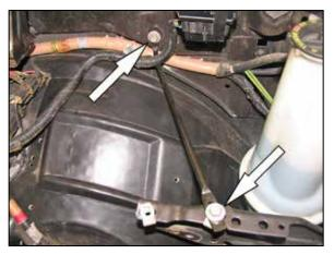
8. Remove the two bolts, which secure the support rod to the inner fender and to the core support, then remove the support rod from the vehicle.
