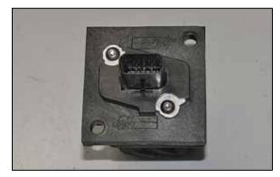
13. Install the mass air sensor into the mass air adapter plate and secure with the factory mounting screws as shown.
