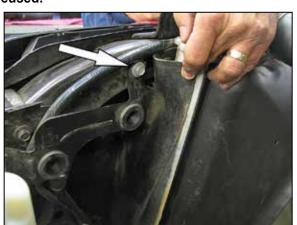
10. Remove the upper air box mounting bracket bolt shown.
