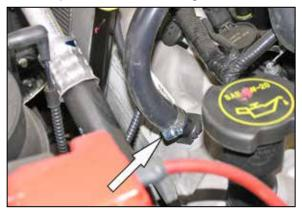
28. Install the provided crank case vent hose onto the valve cover port and secure with the provided hose clamp.
