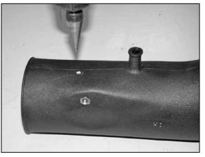
19. On vehicles equipped with an air temp sensor. Drill a 5/8" hole at the drill point indicated on the K&N<sup>®</sup> intake tube.
