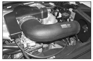
23. Install the new  $K\&N^{\otimes}$  intake tube onto the silicone hose.
