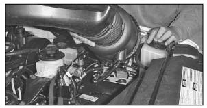
6. Detach the stock intake tube from the throttle body and lift up on the air cleaner assembly to release it from it's retaining grommets. 8. Remove the entire stock intake assembly. NOTE: K&N Engineering, Inc., recommends that customers do not discard factory air intake.
