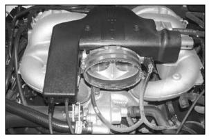
21. Install the silicone hose (08623) onto throttle body with provided hose clamps as shown.
