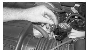
3. On vehicles equipped with air temp sensor, disconnect wire connector from air temp sensor.
