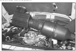
2. Unhook and remove speed control cable and throttle cable from the stock intake tube.
