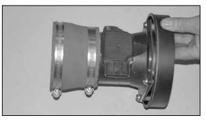
27. Install the silicone hose (08050) onto the mass air assembly with provided hose clamp as shown.
