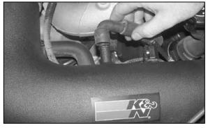
25. Install the air temp sensor into the K&N<sup>®</sup> intake tube, reconnect the air temp electrical connection and install crank case vent onto the vent port.
