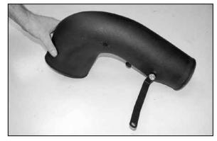
22. Install the provided bracket (07169) onto the K&N^ ${\ensuremath{\mathbb S}}$  intake tube with hardware provided.
