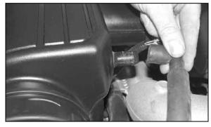
4. Disconnect crank case vent from stock intake tube.
