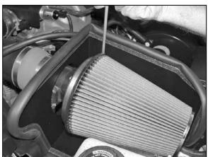
30. Install the K&N<sup>®</sup> air filter onto the mass air sensor and secure it with the provided hose clamp. NOTE: Drycharger<sup>®</sup> air filter wrap; part # RC-5046DK is available to purchase separately. To learn more about Drycharger<sup>®</sup> filter wraps or look up color availability please visit http://www.knfilters.com<sup>®</sup>.
