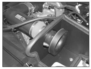
28. Install the mass air sensor assembly onto the new intake tube as shown.
