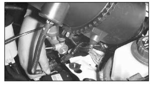
7. Disconnect the secondary mass air sensor electrical connection.
