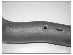
12. Install the crank case vent grommet into the K&N® intake tube as shown.
