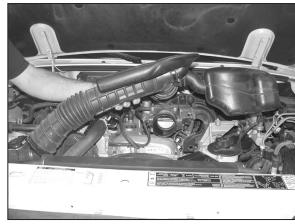
6. Loosen the hose clamps at the throttle body and the mass air sensor, then remove the intake tube as shown.
