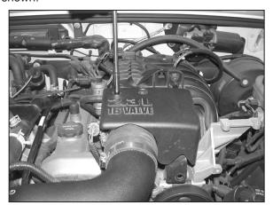
23. Re-install throttle body cover removed in step
