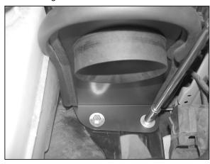
18. Install the mass air assembly onto the air box mounting bracket and secure with the provided 3/8" bolts.
