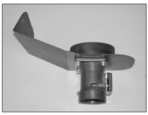
14. Assemble the mass air adaptor, heat shield, gaskets and the mass air sensor as shown using the provided hardware.
