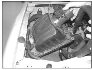
7. Unhook air filter lid clips and remove air filter lid assembly, as shown.
