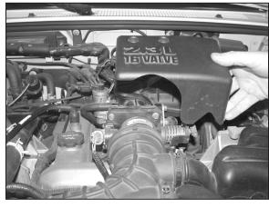
4. Remove the two 7mm screws that secure the throttle body cover then remove the throttle body cover.
