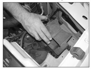
9. Pull firmly on the air inlet duct to release the duct from the radiator core support as shown.
