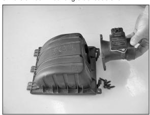
11. Loosen and remove the four hex bolts that secure the mass air sensor, then, remove the mass air sensor from the air box lid.
