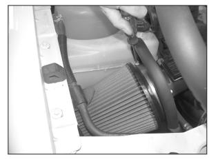
19. Install the K&N® filtercharger onto the mass air assembly as shown.
