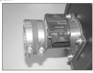
16. Install the silicone hose (08190) onto the mass air sensor with the provided hose clamps as shown.
