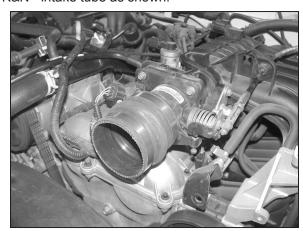
13. Install the provided silicone hose (08696) onto the throttle body with provided hose clamps as shown.
