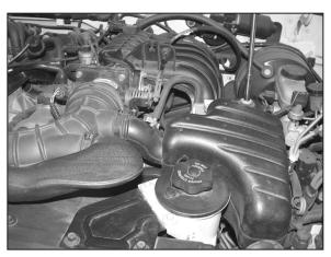
5. Vehicle's equipped with resonator chamber on intake tube, remove the 8mm bolt that secures resonator to mounting bracket.
