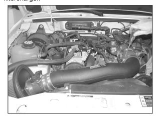
21. Install the K&N® intake tube onto the mass air assembly and then onto the throttle body as shown.
