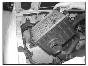
8. Slide a flat blade screwdriver in between the airbox and the airbox mounting tray. Pry downwards on the tray, while pulling upwards on the airbox assembly to release the assembly from the retaining grommets in the tray.
