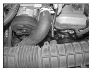
3. Disconnect crank case vent from intake tube as shown.
