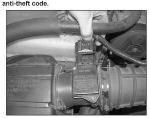
2. Disconnect the mass air sensor electrical connection, then disconnect wiring harness from intake tube.
