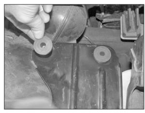
17. Install the two provided nut inserts into the air box mounting bracket as shown.
