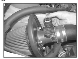
24. Reconnect the mass air sensor electrical connection and secure wire harness in retaining clips onto intake tube.
