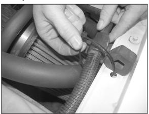
20. Using the provided tie wrap, secure the coolant recovery hose to the inner fender about the K&N® filtercharger.
