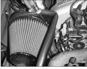
15. Install the air filter onto the adapter and secure it with the hose clamp provided.
