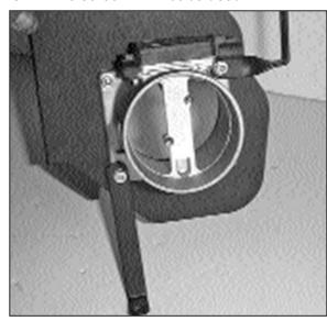
8. Assemble the mass air sensor, adapter, gaskets, heat shield and brackets using the hardware provided.
