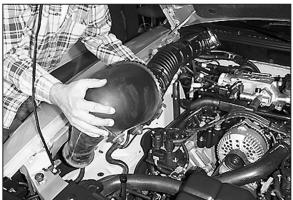
8. Remove the entire air intake assembly. Note: K&N recommends that customers do not discard factory air intake.
