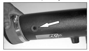
19. On models equipped with an external air temp sensor install the grommet into the hole in the previous step.
