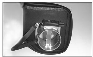
15. Attach the brackets to the mass air sensor as shown.
