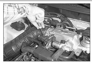
4. Loosen the hose clamp on the intake tube at the throttle body.
