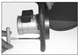
14. Assemble the mass air sensor, heat shield and adapter, using the gaskets and hardware provided as shown.
