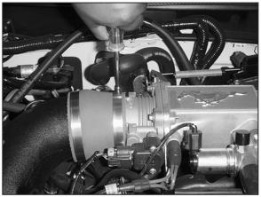
25. Secure the silicone step hose to the throttle body using the hose clamp provided.
