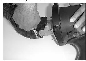
9. Loosen the hose clamp and detach the intake tube from the mass air sensor.
