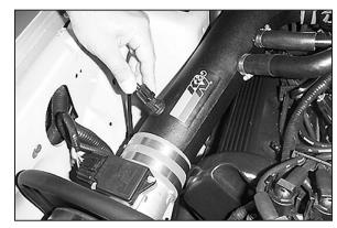
30. Reconnect the mass air sensor and air temperature sensor electrical connections. NOTE: Not all models are equipped with an external air temp sensor.
