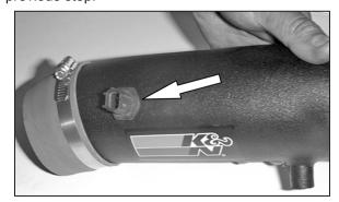
20.On models equipped with an external air temp sensor, insert the air temperature sensor into the grommet.
