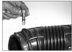
10. On models equipped with an external air temp sensor remove the air temperature sensor from the intake tube.
