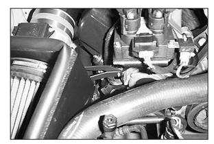
26. Secure the brackets to the protruding stud using the hardware provided.
