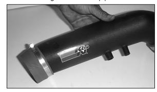
17. Attach the silicone straight hose (08630) to the  $K\&N^{\odot}$  intake tube using the hose clamp provided.
