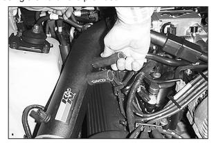
27. Attach the 5/8" and 3/4" ID vent hose provided onto the appropriate vent fittings on the intake tube using the hose clamps provided.
