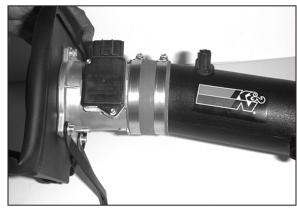
21. Attach the K&N $^{\odot}$  intake tube to the flange on the mass air sensor using the hose clamp provided.
