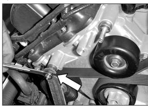
23. Loosen and remove the nut from the protruding stud on the engine.
