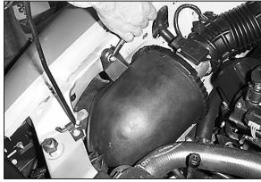
5. Loosen and remove the bolt that retains the air cleaner.
