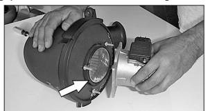
12. Remove the mass air sensor from the air cleaner.
