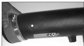
18. On models equipped with an external air temp sensor, drill out the drill point using a 11/16" drill bit.
