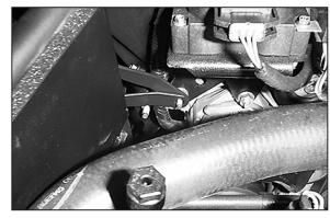
24. Install the K&N® intake assembly, sliding the brackets onto the protruding stud on the engine as shown above.
