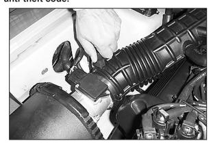
2. On models equipped with an external air temp sensor, disconnect the air temp sensor electrical connection.
