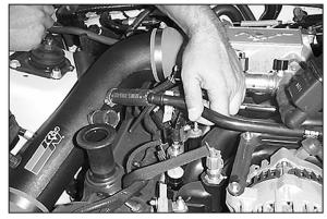
28. Install the PCV line into the 3/4" ID vent hose.
