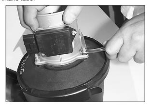
11. Loosen and remove the 4 nuts that retain the mass air sensor.
