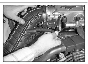
7. Detach the PCV line from the intake tube.
