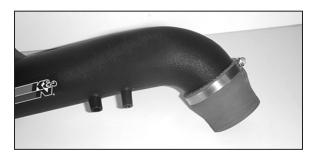
16. Attach the silicone step hose to the K&N<sup>®</sup> intake tube using the hose clamp provided.
