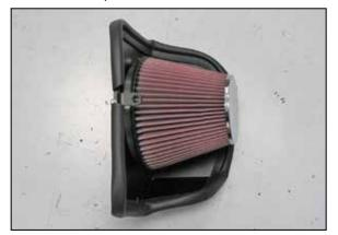
12. Install the K&N<sup>®</sup> air filter onto the filter adapter and secure with the provided hose clamp. NOTE: Drycharger<sup>®</sup> air filter wrap; part # RF-1048DK is available to purchase separately. To learn more about Drycharger<sup>®</sup> filter wraps or look up color availability please visit http://www.knfilters.com<sup>®</sup>.
