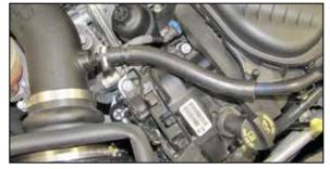
20. Install the factory quick disconnect fitting into the provided crank case vent hose and then install the assembly onto the factory hardline and connect the quick disconnect fitting to the fitting installed into the K&N<sup>®</sup> intake tube.
