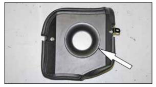
11. Install the filter adapter into the heat shield and
