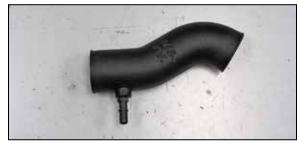
15. Install the provided quick disconnect fitting into the K&N $^{\odot}$  intake tube as shown.
