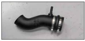
16. Install the provided hump coupler (5-576) all the way onto the K&N $^{\odot}$  intake tube but do not secure at this time.
