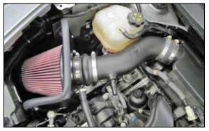
17. Install the K&N<sup>®</sup> intake tube into the coupler at the intake plenum and then slide the hump coupler onto the filter adapter. Adjust the intake tube for best fit and then secure with the provided hose clamps and heat shield mounting hardware.
