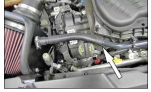
18. Remove the flexible crank case vent line from the hard line.
