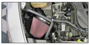
13. Install the heat shield assembly into the vehicle and secure with the hardware removed in step #6. **NOTE: Do not completely tighten at this time.**
