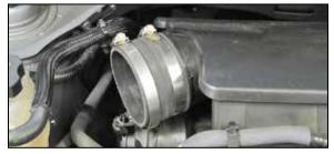
14. Install the provided coupler hose (08690) onto the intake plenum and secure with the provided hose clamp.
