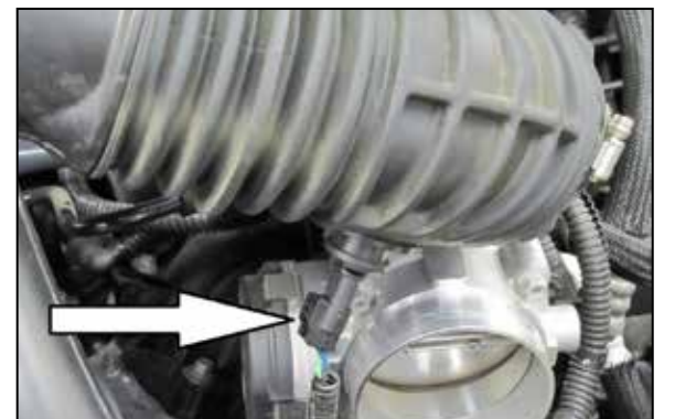
6. Lift up the intake tube, disconnect the inlet air temperature electrical connection then remove the intake tube from the vehicle.
