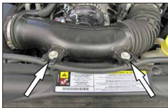
3. Remove the two bolts which secure the factory intake tube to the fan shroud.
