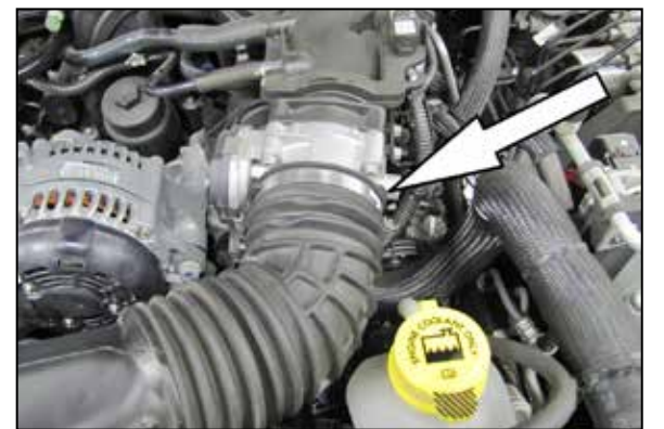
5. Loosen the hose clamp securing the factory intake tube to the throttle body.
