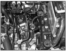
13. Install the rubber mounted stud into the center air box mounting location as shown.
