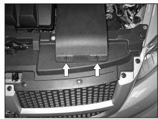
2. Unlock the two fresh air retaining clips by turning a ¼ turn counter clockwise.
