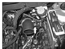
21. Attach the remaining vent hose to the 1/4NPTx3/8" vent fitting installed in the K&N® intake tube.
