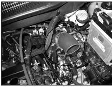
19. Install the K&N® intake tube into the silicone hose at the turbo inlet and align with the mounting bracket, then secure with the provided hose clamps.
