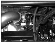
15. Install the provided silicone hose (08095) onto the turbo inlet and secure it with the provided hose clamp.
