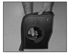
23. Install the provided edge trim into the hole of the heat shield as shown.
