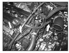
20. Install the provided crank case vent hose to the 1/4NPT X 1/2" on the K&N® intake tube and then attach the other end to the vent port on the valve cover as shown.
