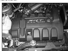
26. Reinstall the engine cover onto the valve cover.
