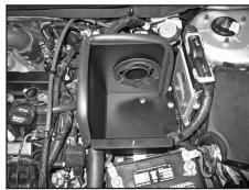
24. Install the heat shield onto the rubber mounted stud installed during step #13 and onto the ECU mounting studs. Then secure the heat shield with the factory ECU mounting bolts and hardware provided.
