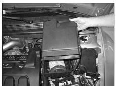
5. Unhook the upper air box retaining clips and then remove the upper air box as shown.
