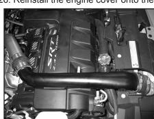
27. Reinstall the intercooler tube and secure with the factory hose clamps.
