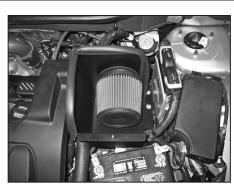
28. Install the K&N® air filter onto the intake tube and secure with the provided hose clamp.
