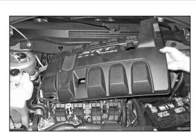
7. Lift up the engine cover to dislodge it from the mounting studs and then remove the engine cover from the vehicle.
