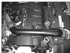
6. Loosen the two hose clamps that secure the intercooler transition tube. Then remove the intercooler transition tube.
