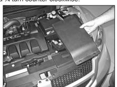
3. Remove the fresh air intake scoop from the vehicle.
