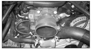
9. Install the supplied silicone hose onto the throttle body and secure with the supplied hose clamp.
