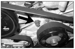
10. Remove the front engine bolt shown. **NOTE: This bolt will be reused.**
