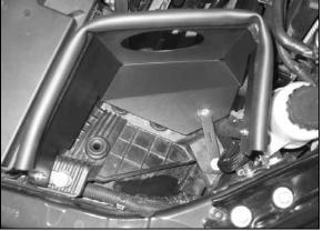
19. Install the heat shield assembly into the engine compartment and secure with the three bolts removed in step #12.
