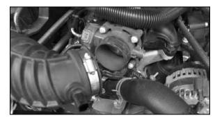
4. Loosen the hose clamp that secures the stock intake tube to the throttle body and then disconnect the intake tube from the throttle body.
