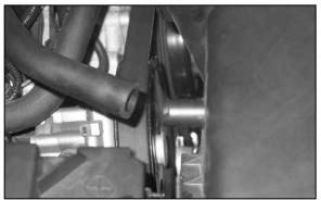
3. Disconnect the crankcase vent hose from the stock intake tube as shown.
