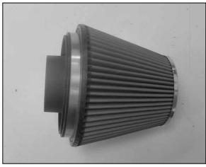
22. Install the air filter adapter into the K&N $^{\otimes}$  air filter and secure with provided hose clamp.
