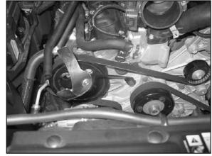
12. Install the tube mounting bracket assembly onto the engine and secure with the bolt removed in step #10.
