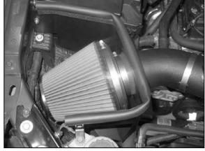
24. Install the K&N<sup>®</sup> air filter assembly on the intake tube and secure with the provided hose clamp as shown.
