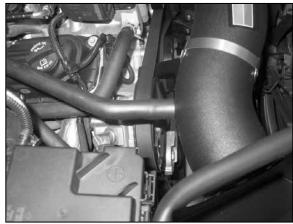
21. Connect the crankcase vent hose to the intake tube.
