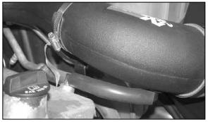
21. Install the provided silicone vent hose onto the valve cover vent and onto the elbow into the K&N $^{\mbox{\ensuremath{\$}}}$  intake tube as shown.
