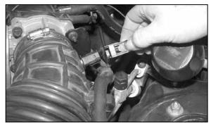
2. Unlock the red locking tab on the air temperature sensor electrical connection, then depress the locking lever and pull apart the temperature sensor electrical connection
