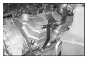
8. Using the provided hardware, install the tubemounting bracket onto the engine at the threaded hole in the cylinder head as shown.
