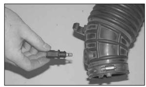
13. Remove the air temperature sensor from the factory intake tube.
