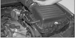
6. Lift the complete intake and air filter assembly to remove it from the vehicle. **NOTE: K&N Engineering, Inc., recommends that**
