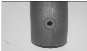
14. Install the provided grommet into the small throttle body end of the intake tube.
