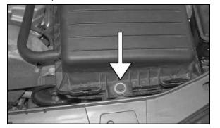
5. Loosen and remove the airbox mounting bolt as shown.
