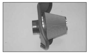
11. Install the K&N $^{\odot}$  air filter onto the filter adapter as shown.
