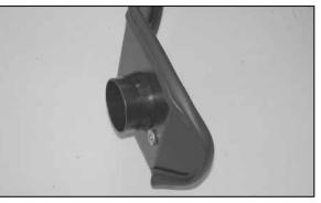
10. Install the air filter adapter onto the heat shield with the provided hardware as shown. NOTE: Be sure to use the rubber gaskets provided.
