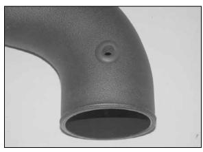
16. Install 2nd supplied grommet into the filter end of the  $K\&N^{\otimes}$  intake tube as shown.
