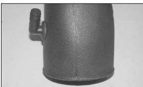
17. Install the provided elbow fitting into the grommet installed instep #16 as shown.
