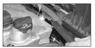
4. Disconnect the crankcase vent hose from the valve cover port as shown.
