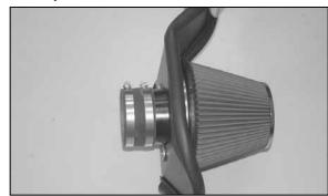
12. Install the silicone hose (08630) onto the filter adapter and secure with the provided hose clamp as shown.
