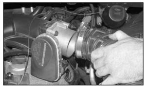
3. Loosen the hose clamp that secures the intake tube to the throttle body and pull the intake tube off the throttle body.
