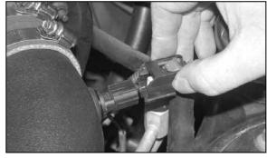
22. Reconnect the air temperature electrical connection as shown.
