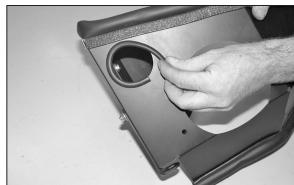
25. Install the edge seal onto heat shield as shown.
