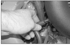
19. Reconnect the intake vent line onto the intake tube, then secure with provided hose clamp.
