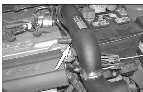
18. Install the K&N $^{\odot}$  intake tube onto the turbo, then align with saddle bracket. Then tighten all hose clamps.
