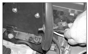
30. Install temp sensor into heat shield then reconnect the electrical connection as shown.
