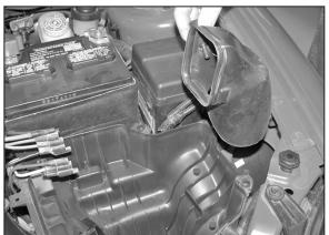
8. Remove the fresh air intake tube from vehicle as shown.
