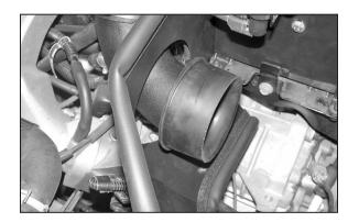
31. Install the filter adapter onto the new K&N® intake tube as shown.
