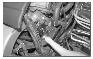
15. Remove the 13mm bolt that secures the engine removal bracket to engine as shown.
