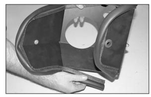
24. Install the edge trim onto the heat shield as shown. Trim if needed.
