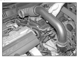
12. Loosen the hose clamp at the turbo, then remove the intake tube as shown.
