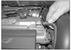
9. Disconnect the crank case vent from valve cover as shown.
