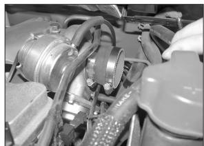
13. Install the provided silicone hose (08284) onto the turbo with the provided hose clamp.
