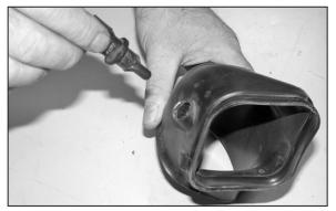
29. Remove temp sensor from fresh air intake as shown.
