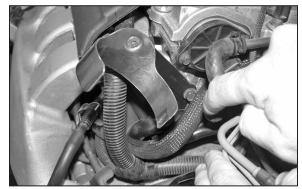
16. Using the bolt that was removed in the previous step, secure saddle bracket assembly onto engine as shown.
