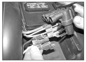
4. Remove the two screws that secure the solenoid pack to air box lid, then disconnect vacuum lines from solenoid pack as shown.
