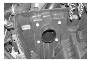
6. Remove the four 10mm bolt that secure the intake tube to air box.
