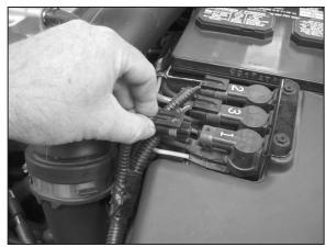
3. Disconnect the three electrical connectors from solenoid pack as shown.
