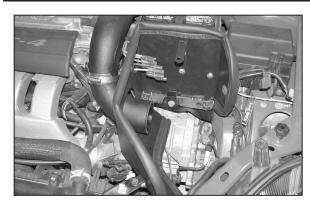
27. Install the heat shield onto vehicle, then secure heat shield to the vehicle with the factory bolts that were removed.
