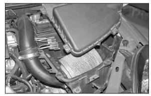
5. Remove the five 8mm bolts that secure the air box lid to air box, then remove lid and air filter as shown.
