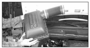
3. Lift up firmly to release the airbox from mounting studs, then remove completely.
