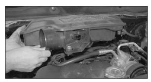
7. Remove the resonator box from vehicle. NOTE: K&N Engineering, Inc., recommends that customers do not discard factory air intake.
