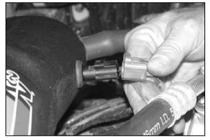
31. Reconnect the air temp electrical connection.
