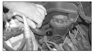
Disconnect the crankcase vent hose from oil fill as shown.
