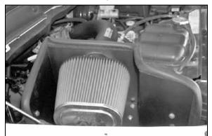
32. Install the K&N $^{\ensuremath{\mathbb{R}}}$  air filter onto the intake tube as shown.
