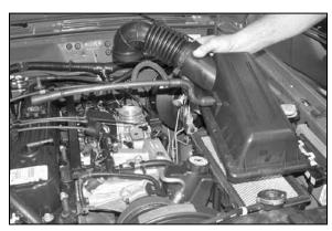
4. Unclip the air box lid, then, remove the upper intake assembly.
