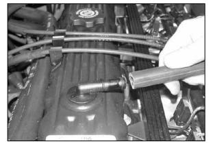
13. Install the provided silicone hose onto the vent on the valve cover.
