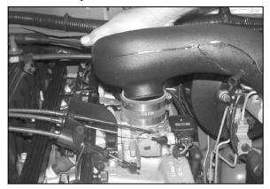
12. Install the K&N<sup>®</sup> intake tube into the silicone hose on the throttle body.
