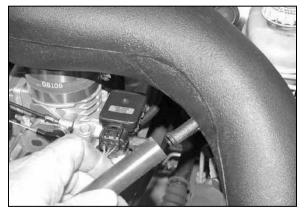
14. Connect the other end of the silicone hose to the vent on the  $K\&N^{\otimes}$  intake tube
