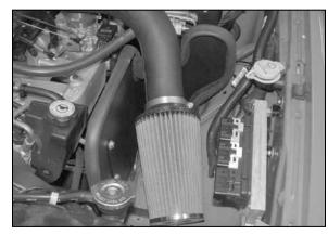
15. Install the K&N $^{\otimes}$  filtercharger onto the K&N $^{\otimes}$  intake tube as shown.
