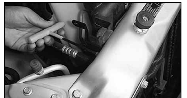
6. Mount the "Z" bracket to the existing hole in the radiator core support.
