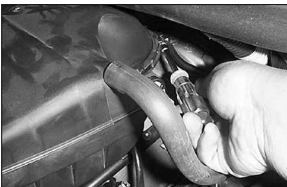
2. Loosen the hose clamp on the air cleaner at the throttle body.
