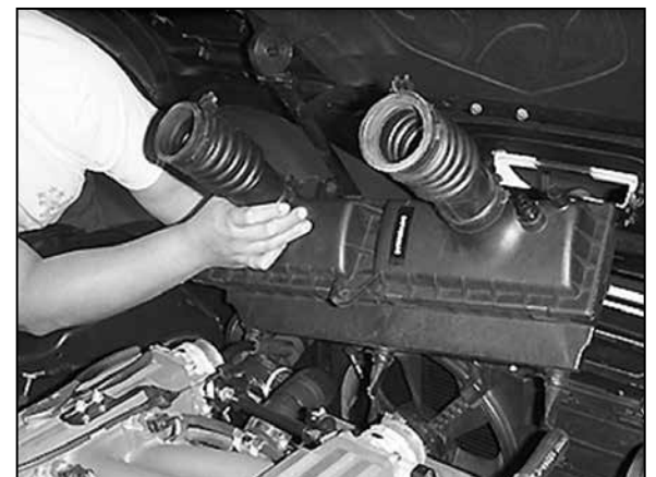
7. Remove the air box assembly. NOTE: K&N Engineering, Inc., recommends that customers do not discard factory air intake.
