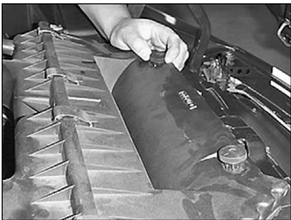
2. Loosen the three air box retaining screws, two in front and one in rear.
