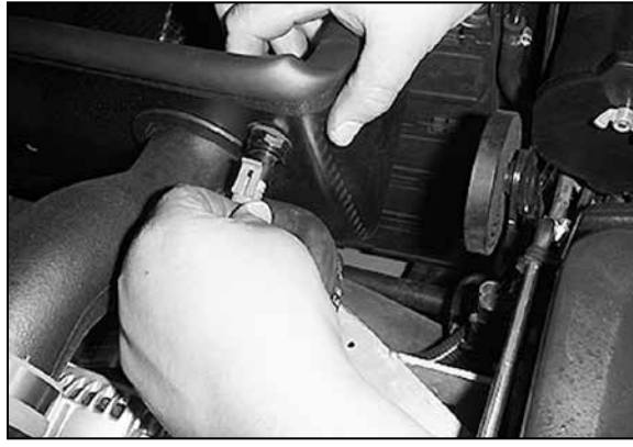
29. Reconnect the air temperature electrical connection.
