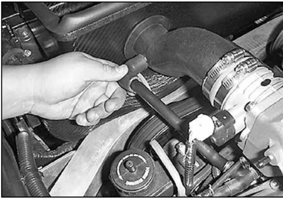
27. Using the vent hose provided, connect the vent tube to the vent on the intake tube.
