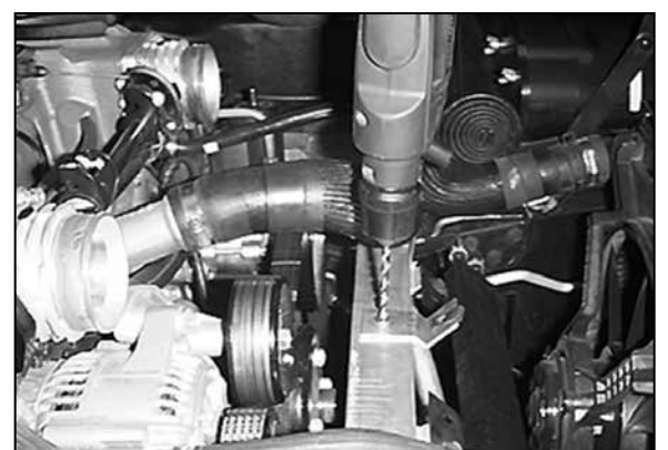
9a. On models equipped with an aluminum crossmember, drill out the rivet that retains the rear air box mounting bracket. Remove the bracket as it will not be used.
