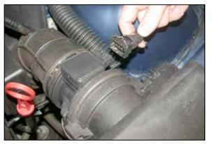
2. Depress the wire-locking clip and disconnect the mass air sensor electrical connection.
