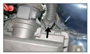
7. Unhook the wiring harness from the rear of the factory air box.
