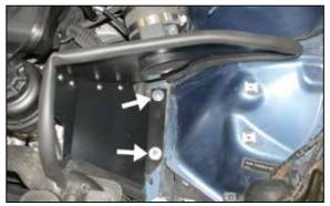
23. Install the heat shield assembly into the vehicle and secure to the lower air box locating studs with the provided hardware as shown. Pass the mass air sensor through the hole in the heat shield.
