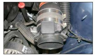
11. Unstrap the heater hose from the lower air box locator, and then pull up to remove the lower air box locator from the vehicle.
