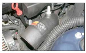
13. Install the K&N<sup>®</sup> intake tube into the factory lower intake hose and secure with the factory hose clamp.
