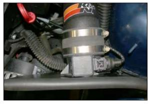
30. Reconnect the mass air sensor electrical connection.
