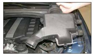
8. Lift up and remove the air box from the vehicle. NOTE: K&N Engineering, Inc., recommends that customers do not discard factory air intake.
