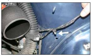
21. Using a pair of pliers, carefully remove the wiring harness retaining clip from the inner fender as shown.
