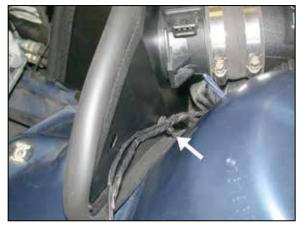
25. Secure the wiring harness clip removed in step #21 to the heat shield as shown.
