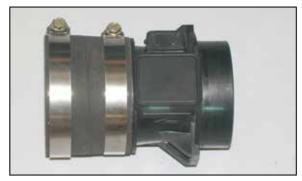
20. Install the silicone hose (08690) onto the mass air sensor and secure with the provided hose clamp.
