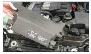
4. Lift up and remove the fresh air duct from the vehicle as shown.
