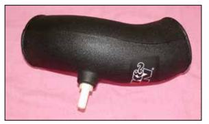
12. Install the provided 1/4" npt fitting into the intake tube as shown.
