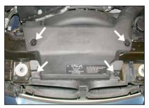
28. Reinstall the fresh air duct removed in step #4 and secure with the four factory retaining pins.
