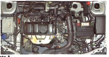
Unclip and remove the breather hose from the air box lid.
