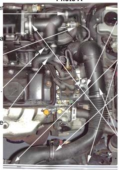
5. Twist and remove the fastener securing the intake pipe to the bracket.
