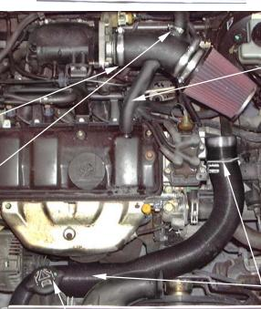
8. Secure the cold air hose to the radiator filler using a long tie ensuring that the hose clears the exhaust and radiator fan.
