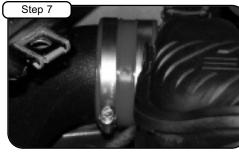
Install the larger 3.25" coupler and clamps on the air box. Do not tighten clamps at this time.
