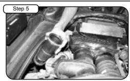
Carefully remove intake tube out of the engine compartment.
