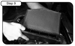
Open the air filter access tray on the side of the air box and remove the OE air filter.
