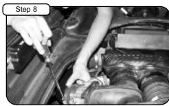
Carefully install the new intake tube in the engine compartment. Tighten all four clamps securing intake tube.
