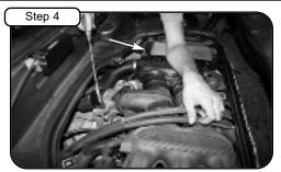
Disconnect hose clamps on both ends of the intake tube.
