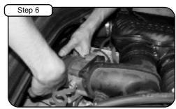
Install the smaller 3" coupler and clamps on the throttle body. Do not tighten clamps at this time.
