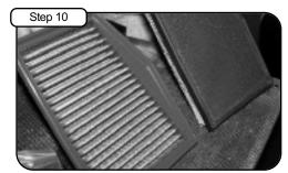
Install the new aFe high flow air filter and reinstall the air filter access tray.
