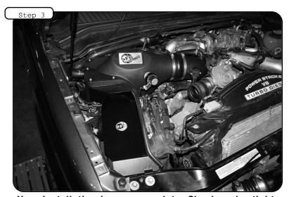
Your installation is now complete. Check and retighten connections and filter after a few hours of operation. Thank You for choosing aFe!
