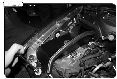
Loosen the 2 bolts near passenger side battery for scoop install using 13mm socket or wrench. Attach trim seal to scoop and allign to cut-out on housing. Reinstall bolts and tighten. Note: Make sure the positive battery terminal is covered with factory cap.
