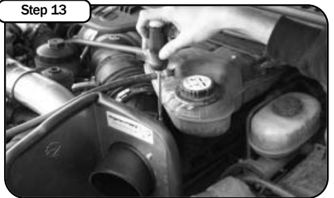
Step 13 Install Factory MAS onto tube using supplied hardware (2 8-32 Screws, 2 nylon spacers, gasket)
