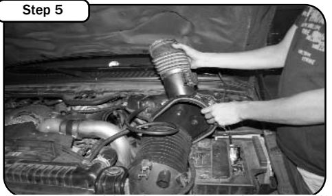
Step 5 Undo the two retaining clips securing the air box outlet. Lift up and remove the turbo inlet tube and filter lid as one piece.
