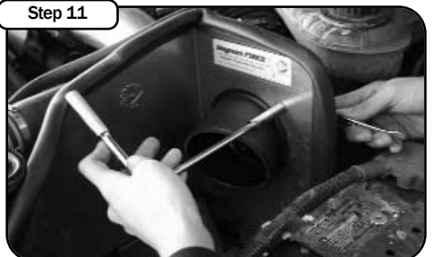
Step 11 Use supplied M6 hardware (2 Screws, 2 Nuts, 2 Wavy Washers) to mount the tube to the housing.
