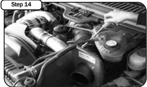
Step 14 Tighten both ends of the factory accordion coupler. Place the included CARB EO Sticker on or near the intake system on a smooth, clean surface. E.O. identification label is required in passing the Smog Check Inspection.
