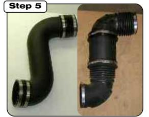
Compare the difference between stock and the Torque Booster Tube. Re-check clamps and connections and retighten after a few hours of operation.
