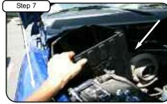
Install housing into vehicle and position.
