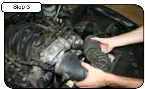
Loosen the clamp at air box side and remove OE intake tube.
