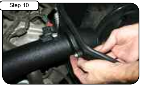
Install screws/nuts and washer provided to mount tube to housing. Tighten using 10mm socket or wrench.
