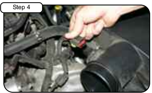
Disconnect MAF sensor harness.
