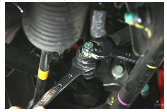
**2b.** Remove the original equipment bushing brackets as well using a **14mm** socket. Note the position of the anti-sway bar in the vehicle to ease in the installation of your new Suspension Techniques Adjustable Anti-Sway Bar. Carefully remove the original equipment anti-sway bar from the vehicle by sliding the end-link out of one side of the bar and pulling the bar out.
