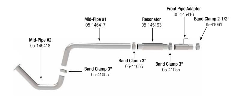
Professional installation is highly recommended. (Read instructions prior to installation). Make sure to always have at least (2) stands or jacks on hand to support the removal of OE system. Also for the installation of aFe system. Any Removal of rubber isolation mounts may require using a spray lubricant such as WD40 and a pry bar.
