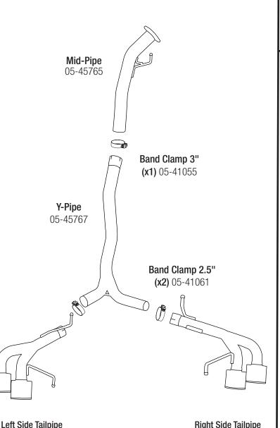
05-45780 Polished Tips 05-45775 Carbon Fiber Tips **Caution:** Allow time for your vehicle to cool down prior to installation. When working on or under your vehicle proceed with caution. Exhaust systems reach high temperatures and may cause serious burns. Wear protective safety equipment; eye goggles and gloves to ensure a safe installation.
