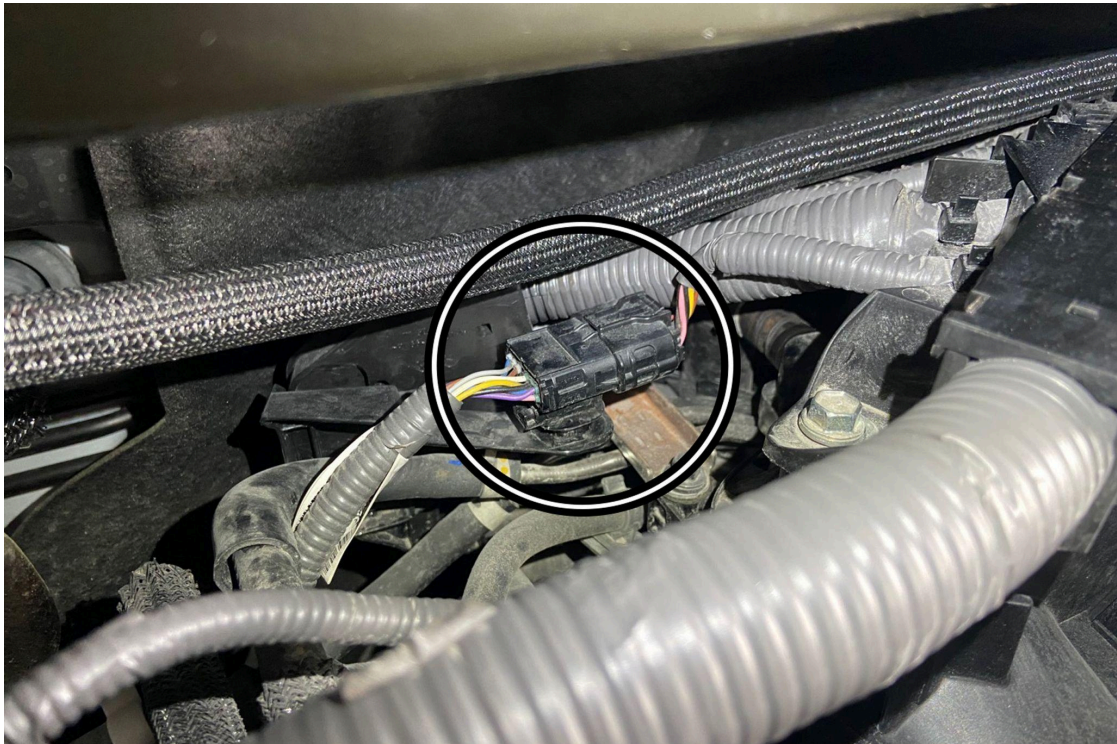
3. Unclip the electrical harness from the mount.
