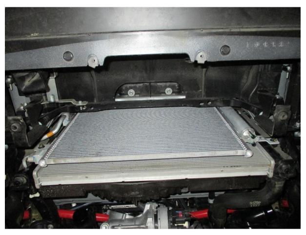
35. Remove the intercooler from the vehicle.
