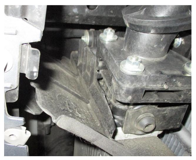
34. Remove the plastic air deflector and intercooler mounting bolt from the drivers side.
