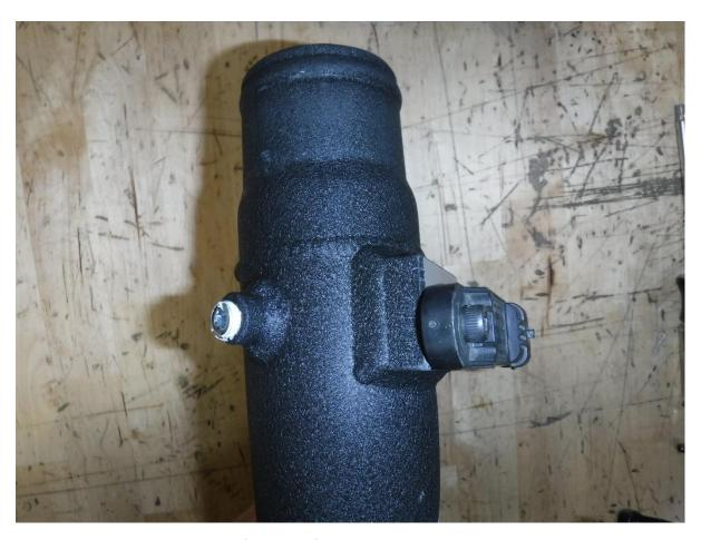
46. Remove the MAP sensor from the factory upper cold side intercooler tube.
