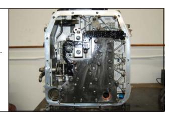
STEP 5. Remove one (1) bolt and remove detent spring.
