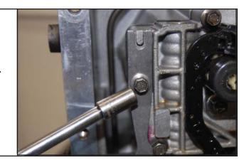
STEP 6. Remove Selector Shaft/Lever Retaining Pin.
