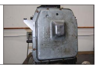
STEP 14. With selector shaft in neutral position, Install Neutral Position Sensor. (NOTE: replace Neutral Position Sensor in same orientation as found before removal). Align sensor to neutral position before tightening two (2) 8mm bolts.
