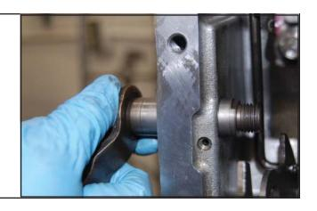
STEP 9. Slide B&M Selector Shaft into case.
