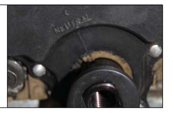
STEP 15. Secure B&M Selector Lever onto B&M Selector Shaft with M10 bolt and M10 washer.
