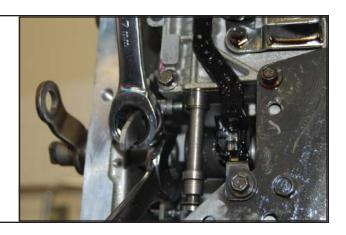
STEP 8. Remove selector shaft from case.
