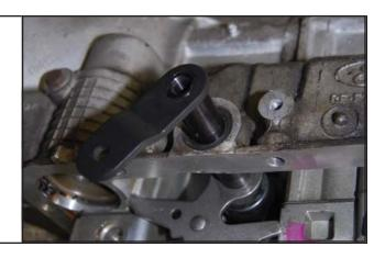
STEP 10. Install Selector Lever Retaining Pin.
