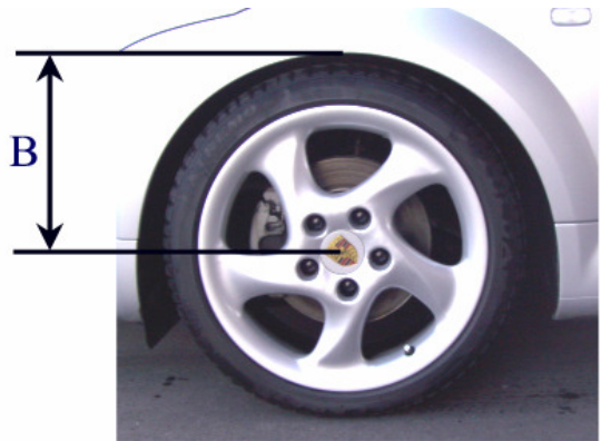
Measurement B Wheel hub center wheel arch
