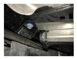
21. Place the reservoir in the bracket, position the reservoir so that the hose does not come in contact with the truck and tighten the hose clamps. Hose clamps can be slid over the outside of the reservoir and should be placed so that they are centered the openings on the bracket.
